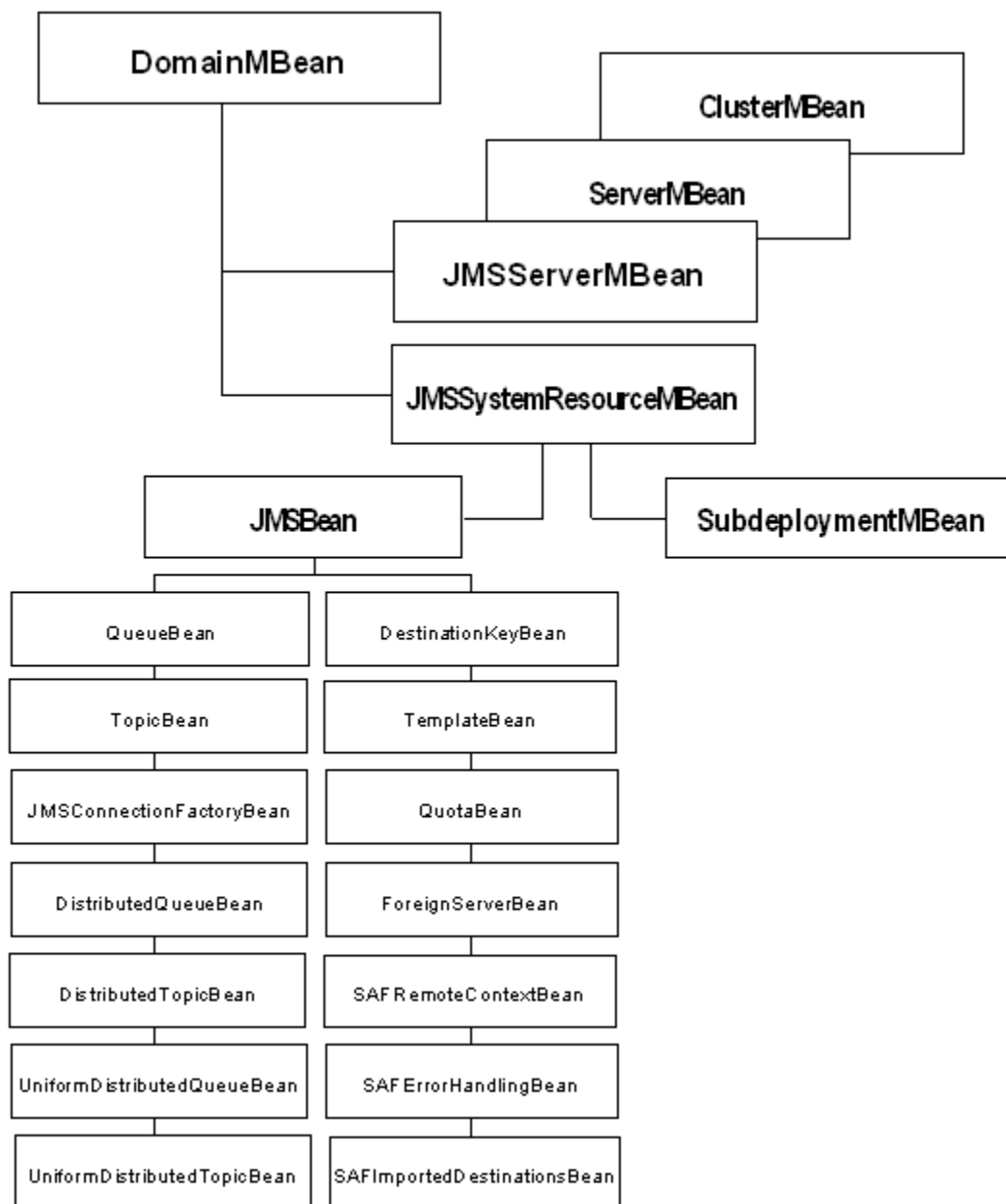
Figure 3-2 JMS Server and JMS System Resource MBeans
