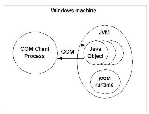
The JVM must call com.bea.jcom.Jvm.register(<jvm id>), where <jvm id> is the id of the JVM as defined in regjvm.
