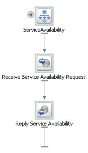
The Start Node contains both a Request variable and a Response variable that were determined by the WSDL operation initially selected. The Receive receives the incoming request message (in this case for the three or fewer different kinds of cable service), and the Reply generates a response message and sends it back to the client.
