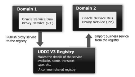
An instance of Service Bus is deployed in each of two domains. The Service Bus proxy service (P1) is configured in domain (D1). The Service Bus proxy service (P2) in domain (D2) requires access to proxy service (P1). As the domains cannot
