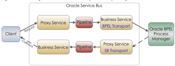
In an asynchronous message exchange, a callback is sent on a different connection than the request.
