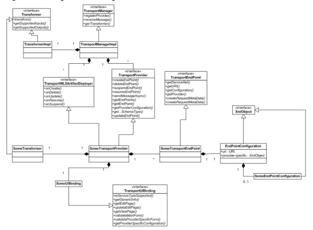
Figure 39-1 Design Time UML Diagram
