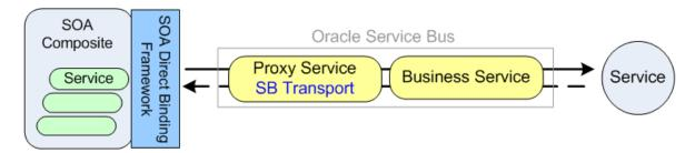
Use the following guidelines to invoke an external service from a SOA composite using direct binding references:
