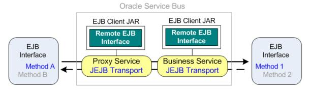
In Figure 30-3, the EJB call is passed through the proxy and business services to invoke another EJB method. Rather than making a direct RMI call outside of Service Bus, this architecture lets you leverage Service Bus features such as message routing, UDDI integration, alerts, monitoring, reporting, and result caching.
