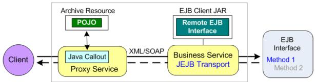
In Figure 30-2, a non-EJB client makes a call to a proxy service configured with a transport that matches the request; for example, a JMS proxy service making an invocation with a JMS topic or queue.
