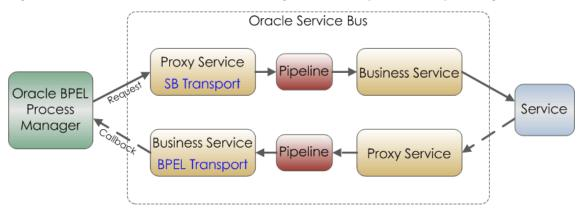
Oracle BPEL Processes Invoking a Service Asynchronously Through Service Bus Figure 34-4
