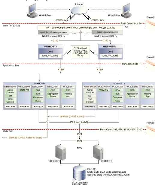
Oracle SOA Suite and Oracle Service Bus Enterprise Deployment Reference Topology Diagram
