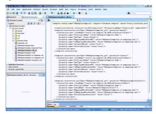
Figure 1-6 Structure of a JCA File
