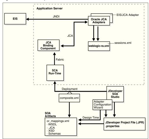
Figure 3-2 Oracle Adapter Architecture in Oracle Fusion Middleware
