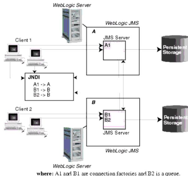
In Figure 2-1, A1 and B1 are connection factories, and B2 is a queue.
