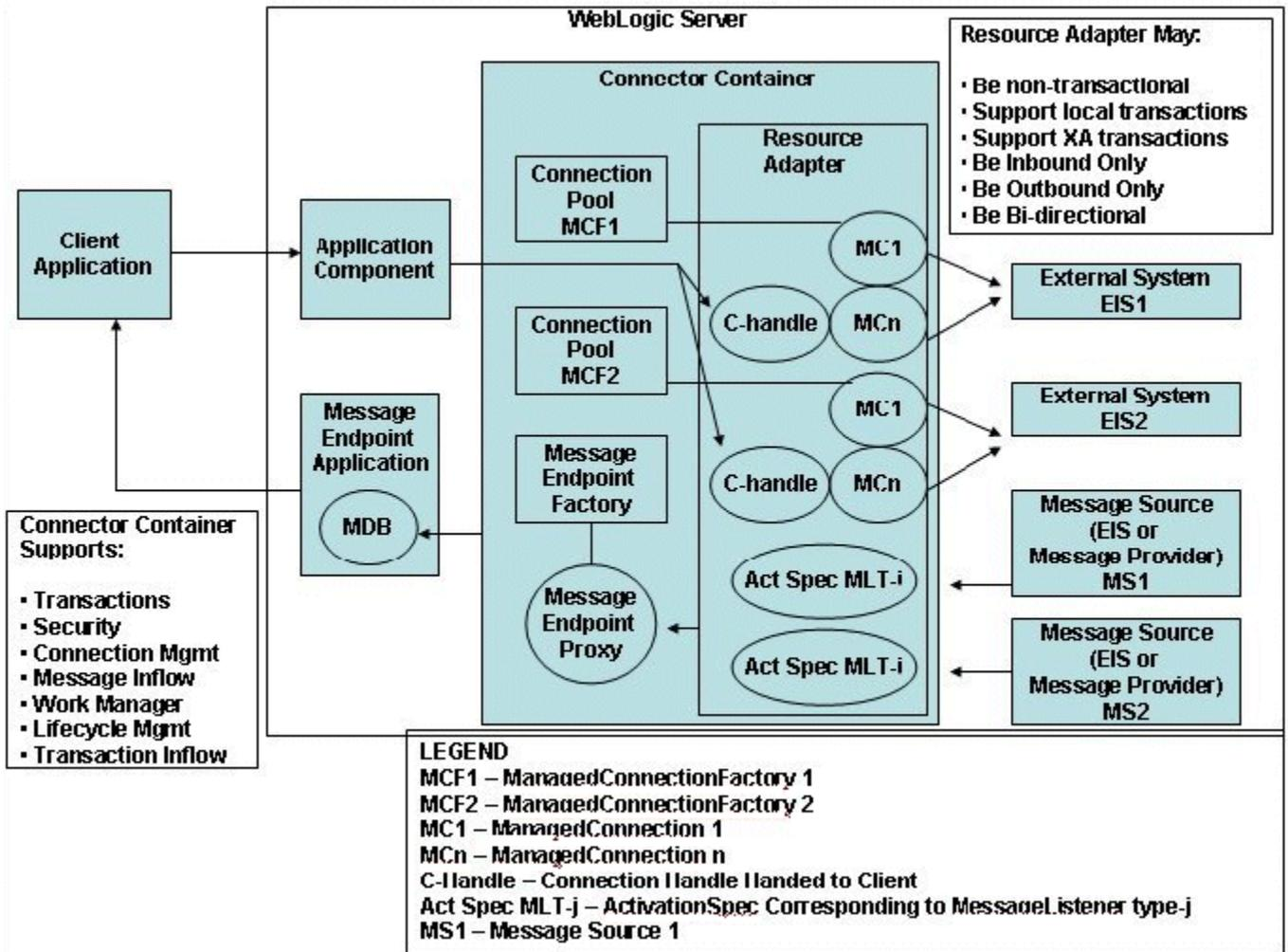
The connector architecture shown in Figure 2-1 demonstrates a bi-directional resource adapter. The following components are used in outbound connection operations:
