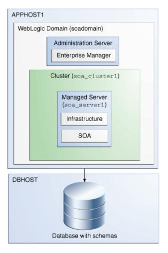
In this topology, Oracle SOA Suite is deployed to the Managed Server.
