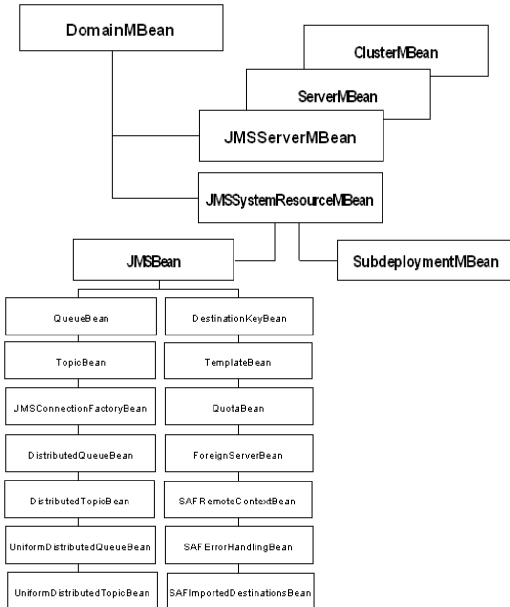
Figure 3–2 JMS Server and JMS System Resource MBeans
