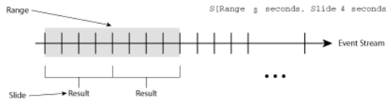
Figure 1-5 Range and Slide: Different (Steady-State Condition)
