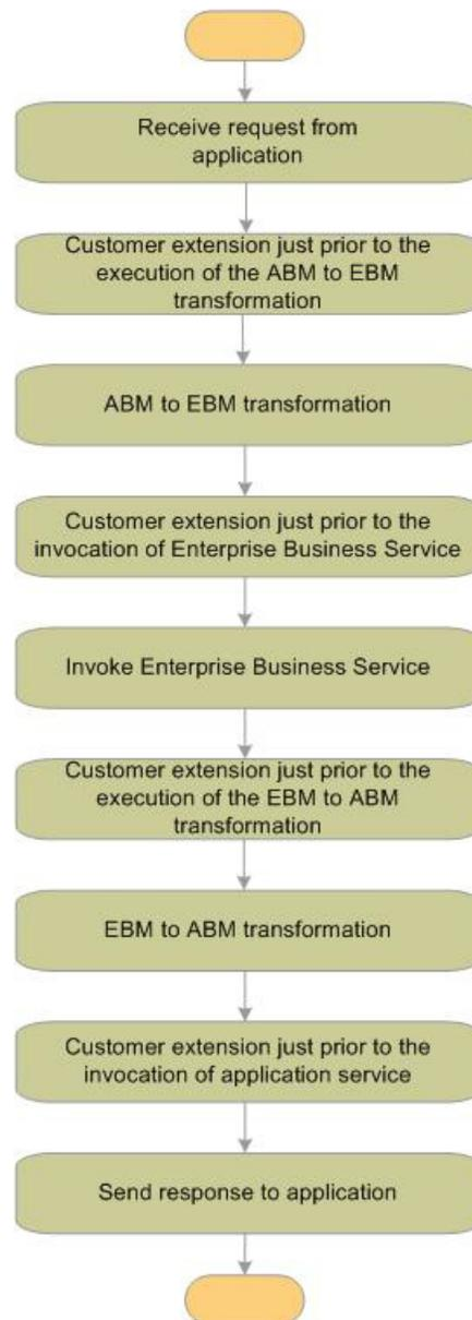
Figure 4–3 depicts the high-level flow of activities in a requester-specific ABCS. The EBS and ABCS interact in a fire-and-forget style. The steps for running the extension to do additional transformations are optional.
