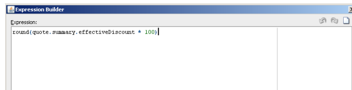
Figure A-55 Expression Used to Change the Value of Discount Project Variable
