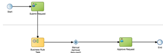
Figure 3–15 The Travel Request Process after Adding the Approval User Task
