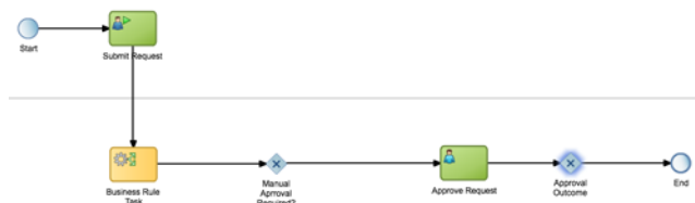
Figure 3–16 The Travel Request Process after Adding an Additional Exclusive Gateway
