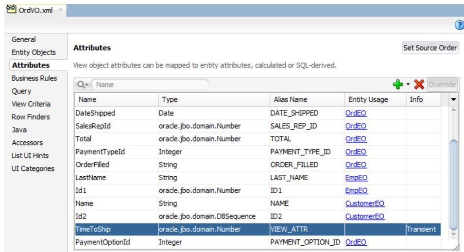
The OrdVO object also contains the TimeToShip transient attribute which is represented by the bars on the ADF Shipping Time bar chart. The TimeToShip attribute’s value is obtained by a call to the calculateTimeToShip() method: `adf.object.calculateTimeToShip(DateOrdered, DateShipped)`. The calculateTimeToShip() method determines the number of days that the order
