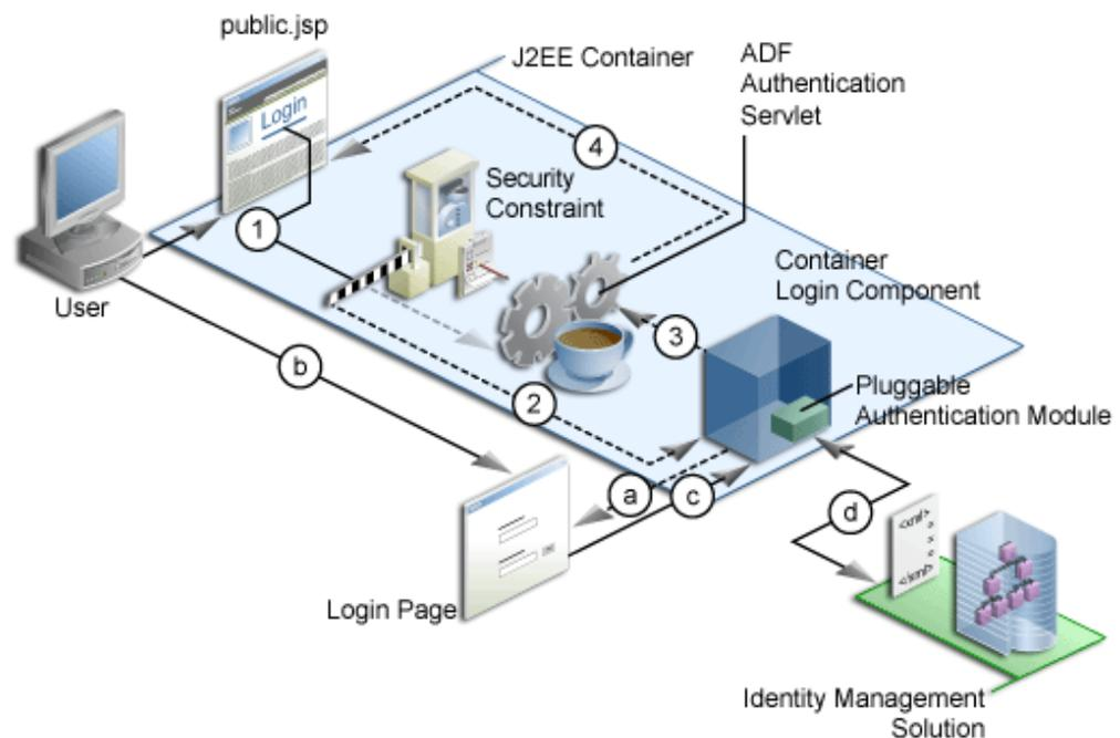
In an explicit authentication scenario, an unauthenticated user (with only the anonymous user principal and anonymous-role principal) clicks the **Login** link on a public page (in the figure, Step 1). The login link is a direct request to the ADF authentication servlet, which is secured through a Java EE security constraint in the web.xml file.
