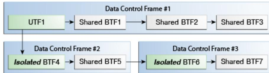
The value that you set for the `data-control-scope` element of a called task flow determines if a calling task flow and a called task flow share flow data controls. Other factors, such as whether a task flow renders in a page or page fragment, do not change this behavior.
