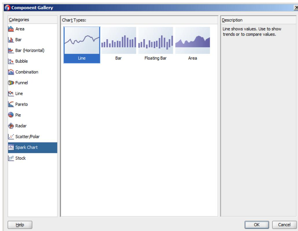
A binding dialog prompts you to specify the value you wish to display for the selected spark chart type. Line, bar, and area spark charts require a single series of data values, for example the changing value of a stock. Floating bar spark charts require two series of data values, one for the float offset, and one for the bar value. For example, in the Create Floating Stacked Bar Sparkchart dialog you specify:
