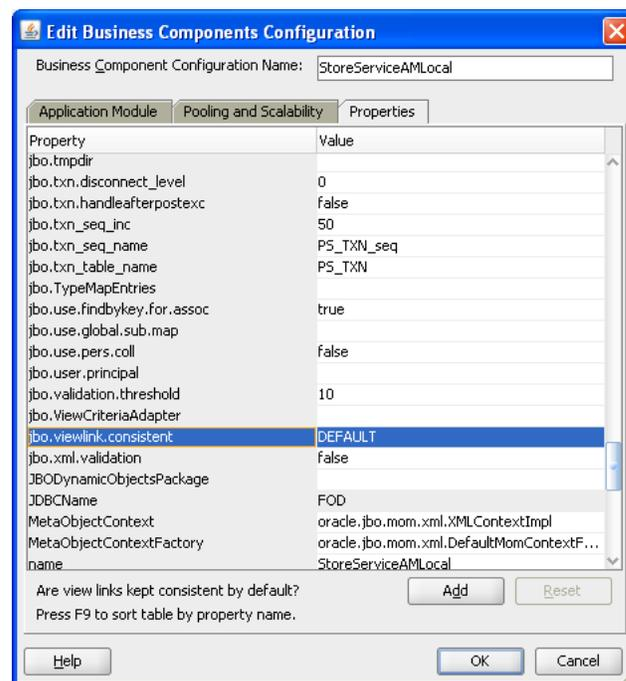
To display the configuration editor, right-click the application module in the Application Navigator and choose **Configurations**. Then, in the Manage Configurations dialog, select the configuration and click **Edit**. In the Edit Business Components Configuration dialog, select the Properties tab. The default setting for this parameter is the word "DEFAULT" which has the following meaning. If your view object has:
