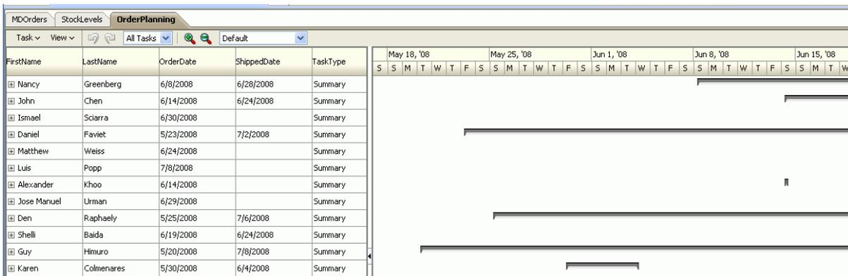
To create a project Gantt chart using a data control, you bind the project Gantt chart component to a data collection. JDeveloper allows you to do this declaratively by dragging and dropping a collection from the Data Controls panel.
