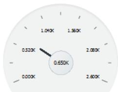
To create a dial gauge using a data control, you bind the gauge component to an attribute in a data collection. JDeveloper allows you to do this declaratively by dragging and dropping an attribute from the Data Controls panel. After you drag and drop the attribute, use the Create Dial Gauge dialog to configure the gauge.
