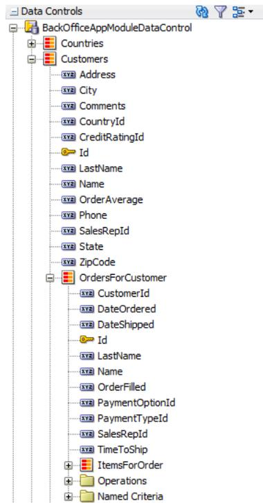
The OrdersForCustomer data control is based on the OrdVO view object. [Figure 26–4](#) shows the OrdVO view object which contains attributes from the OrdEO, EmpEO, and CustomerEO entity objects. The OrdEO, EmpEO, and CustomerEO entity objects are derived from the SOrd, SEmp, and SCustomer tables in the sample application schema.
