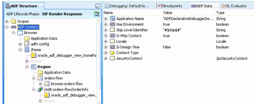
Selecting a view port within the ADF Structure hierarchy will display the view port's current view port details in the ADF Data window, as shown in Figure 31–37. Values displayed for each view port are summarized in Table 31–6.
