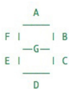
Figure 6-1 Binary Encoding for 7-Segment Display
