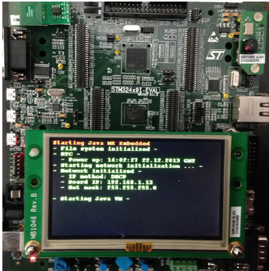
Figure 1-5 The ST Micro STM32429I-EVAL Touchscreen After Installing Java ME Embedded
