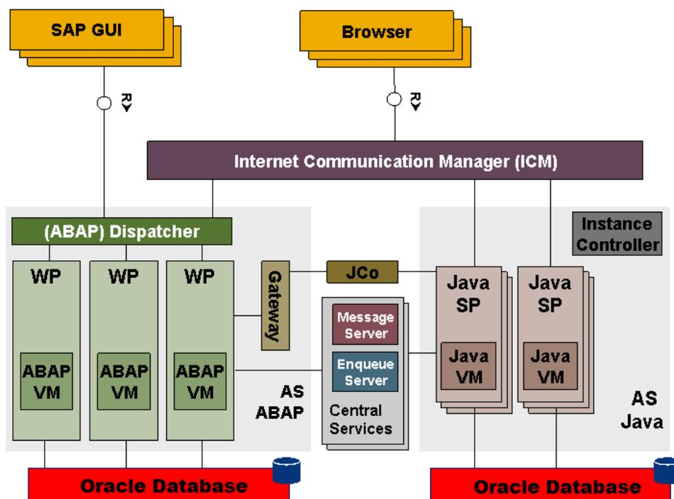
Figure 1: Components of the SAP NetWeaver® Application Server
