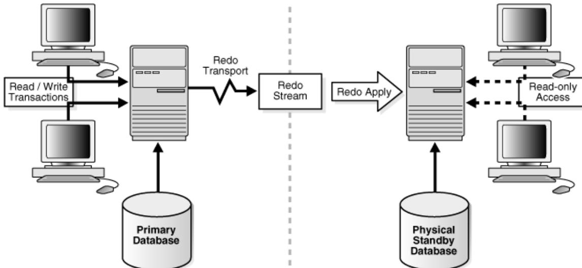
Figure 4: Automatic Updating of a Physical Standby Database
