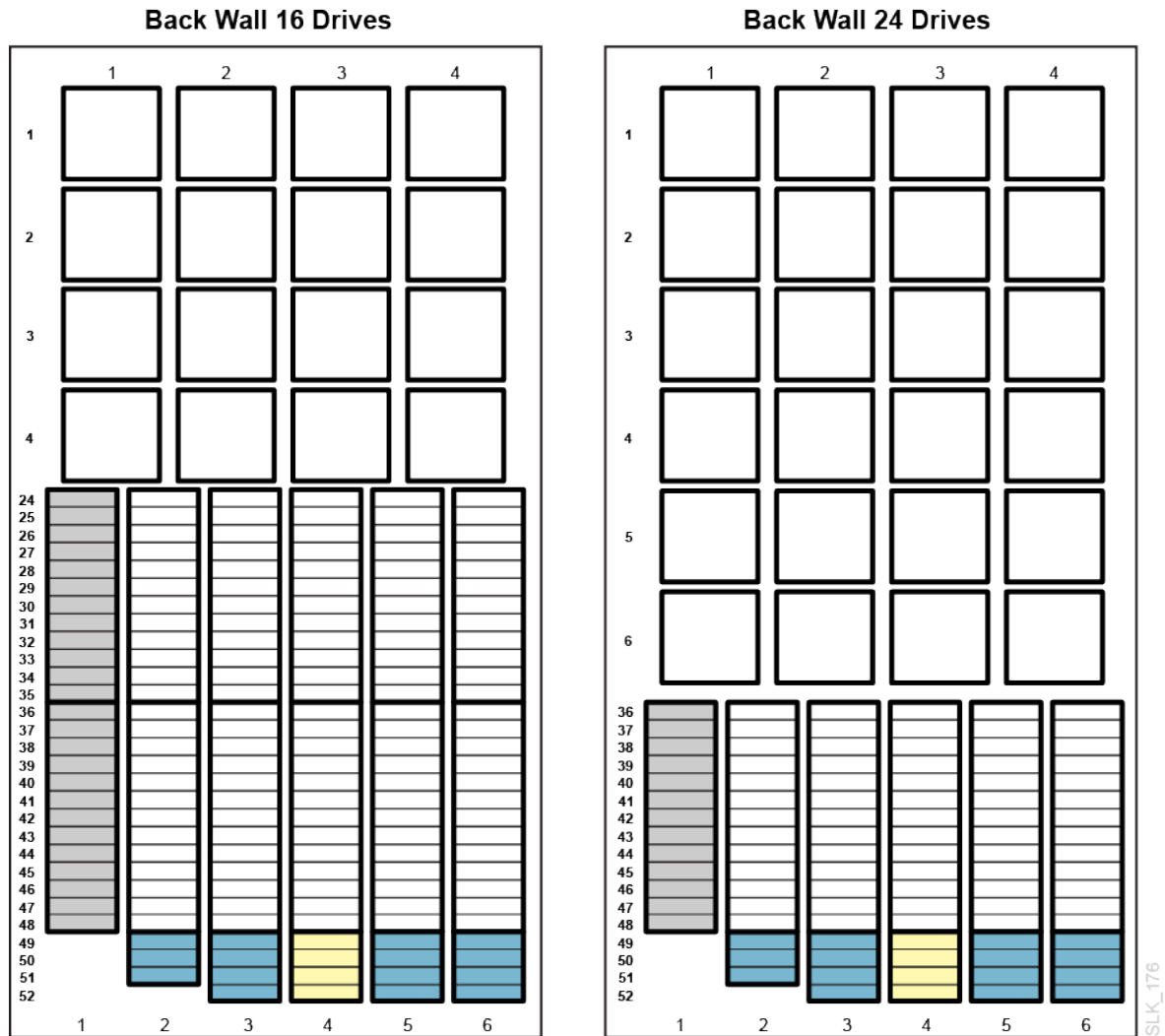
Figure 8-2 Base Module- Back Wall 16 Drives and 24 Drives
