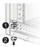
2. Lock the leveling feet, using an 18-mm open wrench.
