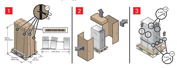
2. Unload the rack from the shipping pallet by attaching the ramps [4], removing the L-brackets [5], and carefully rolling the rack down the ramps [6].
