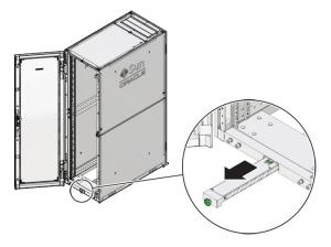
3. Rotate the end of the foot 90 degrees so that it is perpendicular to the floor [1], and adjust the height of the foot so that it rests on the floor [2].
