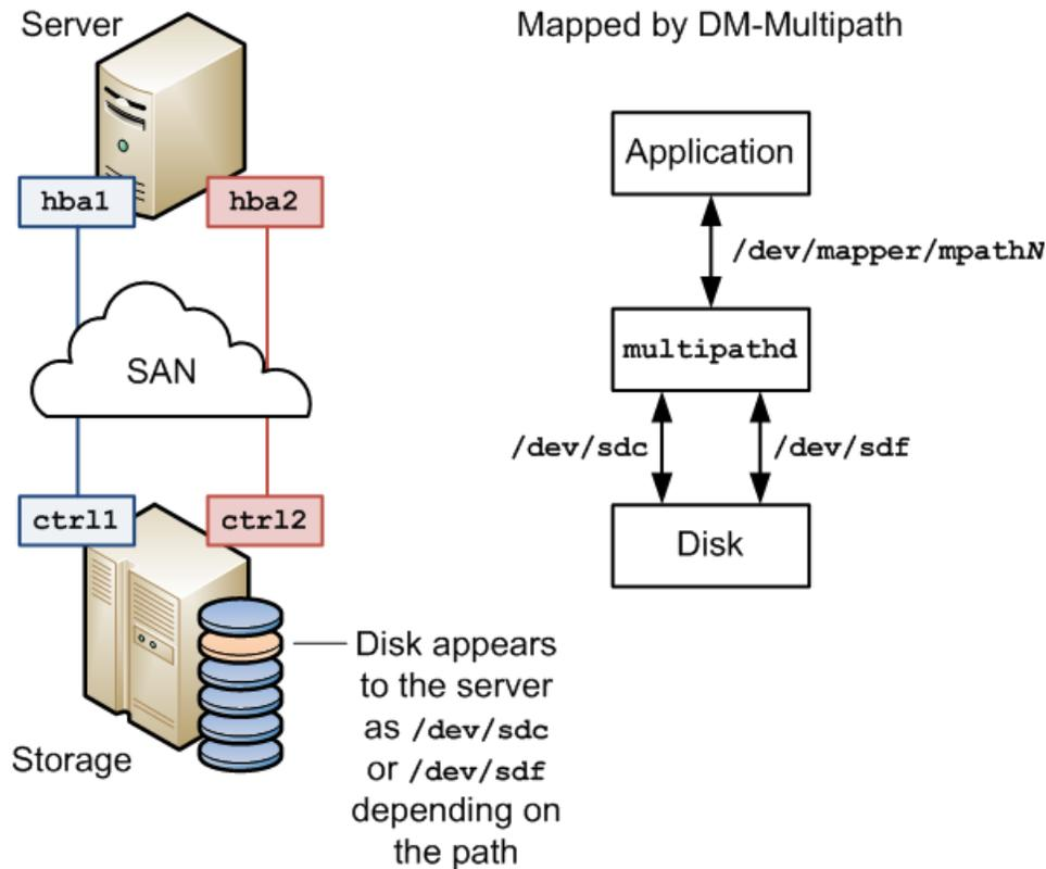
Without DM-Multipath, the system treats each path as being separate even though it connects the server to the same storage device. DM-Multipath creates a single multipath device, `/dev/mapper/mpathN`, that subsumes the underlying devices, `/dev/sdc` and `/dev/sdf`.
