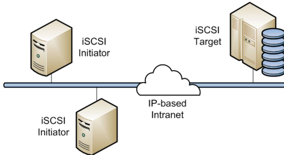
A hardware-based iSCSI initiator uses a dedicated iSCSI HBA. Oracle Linux supports iSCSI initiator functionality in software. The kernel-resident device driver uses the existing network interface card (NIC) and network stack to emulate a hardware iSCSI initiator. As the iSCSI initiator functionality is not available at the level of the system BIOS, you cannot boot an Oracle Linux system from iSCSI storage .
