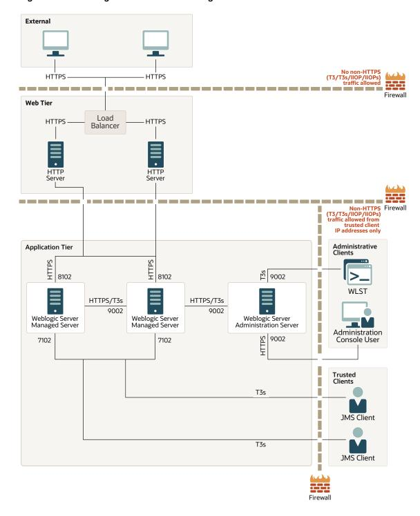
Figure 3-2 WebLogic Server Secure Configuration
