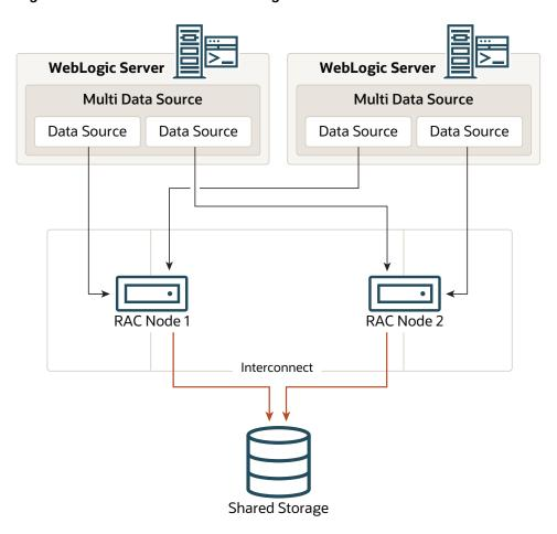
Figure B-2 Multi Data Source Configuration
