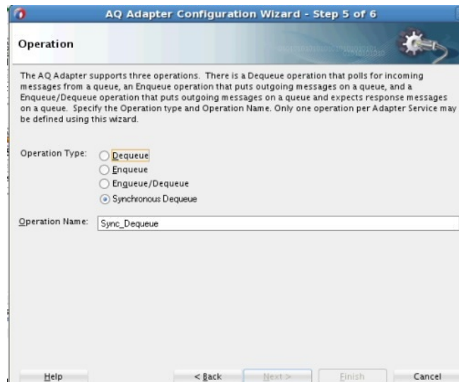
Figure 7-5 AQ Adapter Configuration Wizard Operation Screen with Synchronous Dequeue Operation Selected and Operation Name Sync_Dequeue Shown
