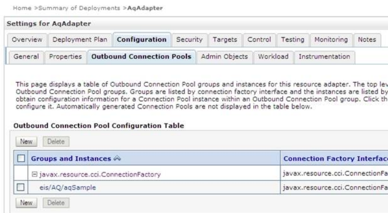
Figure 4-1 Creating Connection Factories using the WebLogic Server Management Console
