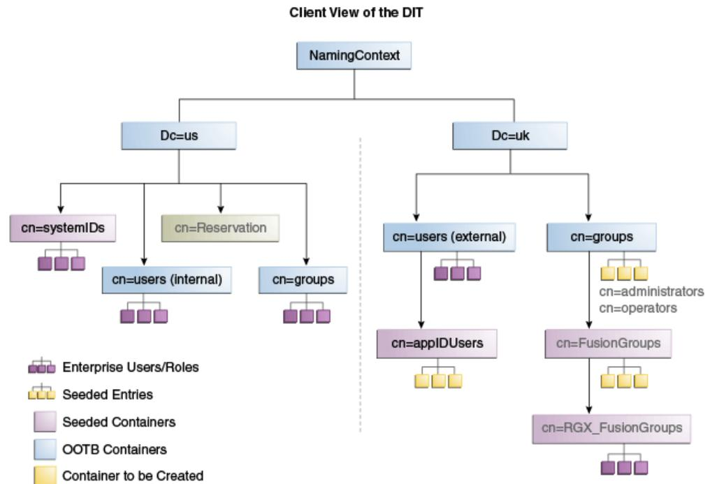
Figure 4-6 provides an overview of the adapter configuration. The classes `inetOrgPerson`, `orclIDXPerson`, and `orclIDXGroup` and the containers `cn=appIDusers` and `cn=fusionGroups` are required only for Fusion Applications.
