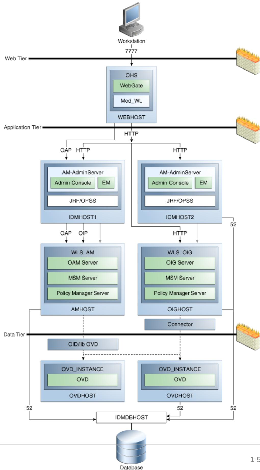
The above diagram shows a basic integration topology where the IdM components Access Manager and Oracle Identity Governance are configured on separate Oracle WebLogic domains:
