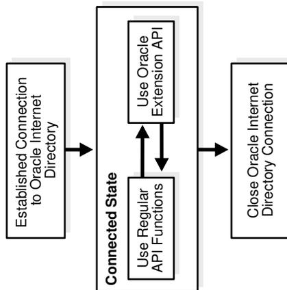
As Figure 4-1 shows, an application first establishes a connection to Oracle Internet Directory. It can then use the standard API functions and the API extensions interchangeably.
