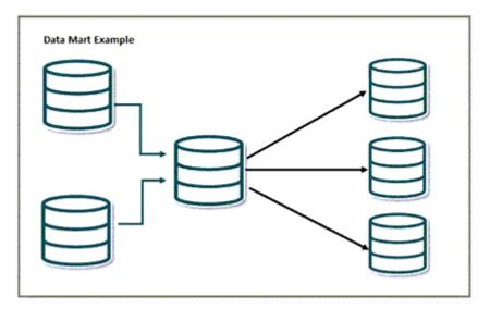
The following image shows central databases that are replicating changes from the Headquarter to the State to the County level in a hierarchical manner.
