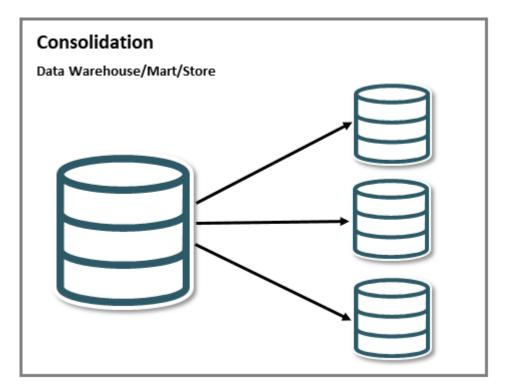
If data is being consolidated into a single target database, it is often necessary to track the lineage of that data. Using Oracle GoldenGate Tokens (link), additional metadata can be written to the target records. This would include the source database information on where this record originated, or when it was committed on the source database.
