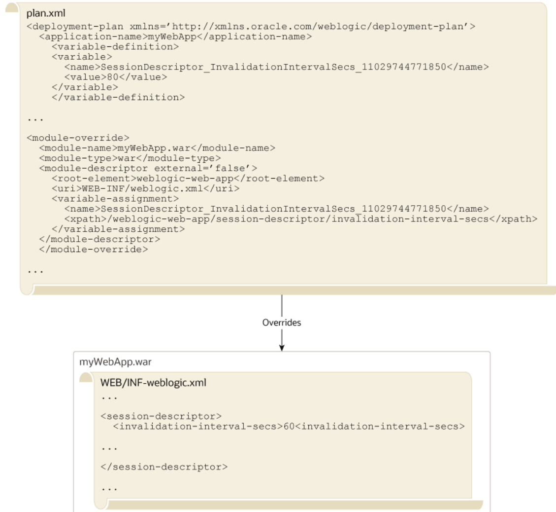
Figure 3-1 WebLogic Server Deployment Plan
