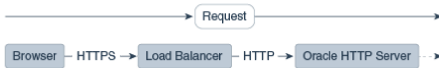
Figure 10-1 Terminating SSL Before Oracle HTTP Server
