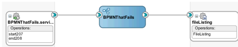
Figure 19-2 Composite with BPMN Process Service Component
