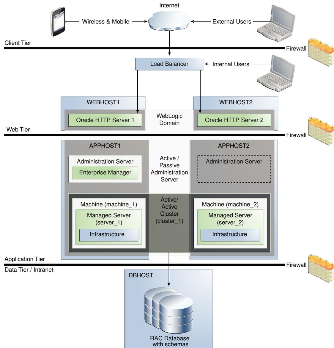
This topology shows a multi-tiered architecture. Users access the system from the client tier. Requests go through a hardware load balancer, which routes them to Web servers running Oracle HTTP Servers in the web tier. Web servers use Proxy Plug-in (`mod_wl_ohs`) to route requests to the WebLogic cluster in the application tier. Applications running on the WebLogic cluster in the application tier then interact with the database cluster in the data tier to service the request.
