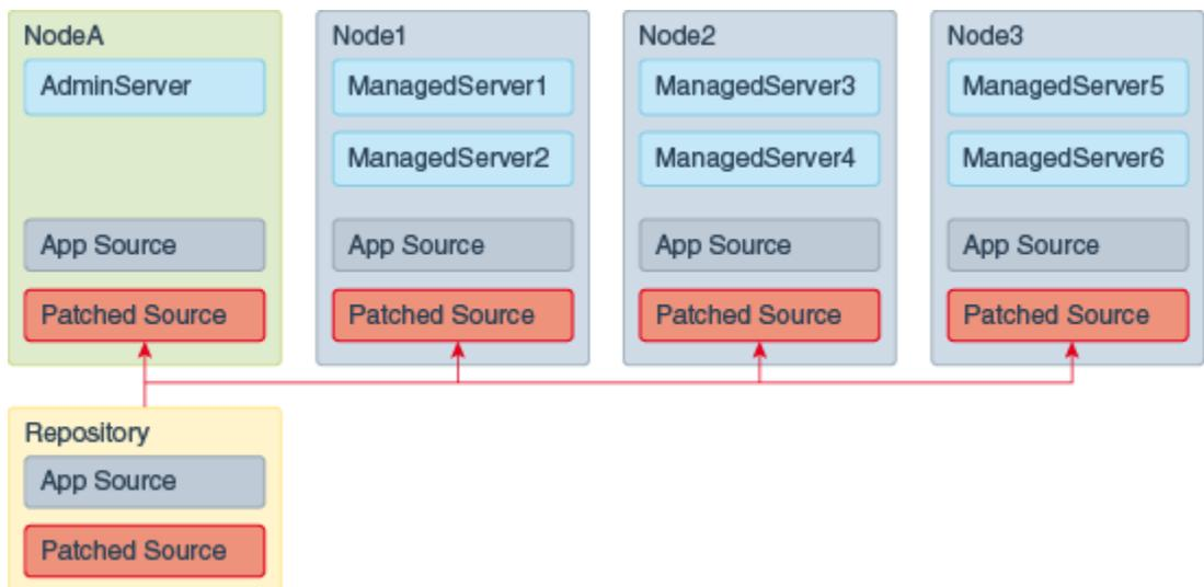
**Figure 1-4 Patching External Staged Applications**
