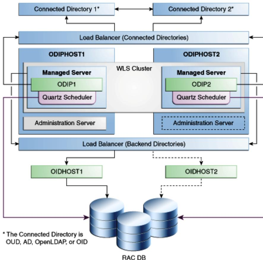
In [Figure 7-2](#), Connected Directory 1 and Connected Directory 2 replicate information with each other. A load balancing router routes requests to the Connected Directories.
