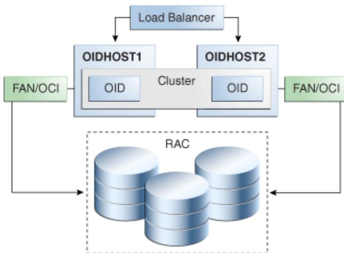
The [Figure 7-1](#) shows Oracle Internet Directory (OID) in the directory tier in a Cluster Configuration high availability architecture. Clustering is set up at installation time. The load balancing router routes LDAP client requests to the two OID instances that are clustered on `OIDHOST1` and `OIDHOST2`.
