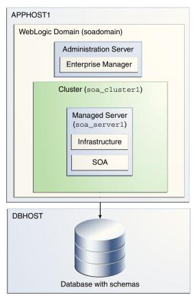
In this topology, Oracle SOA Suite is deployed to the Managed Server.
