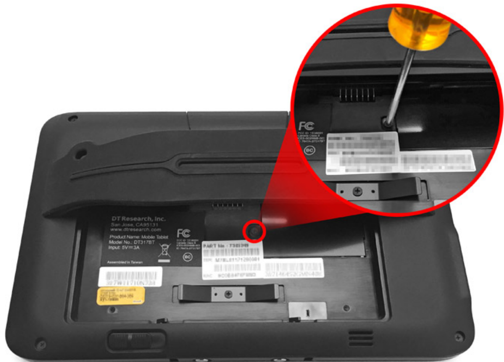
Figure 7-6 Removing the Bridge Battery Cover
