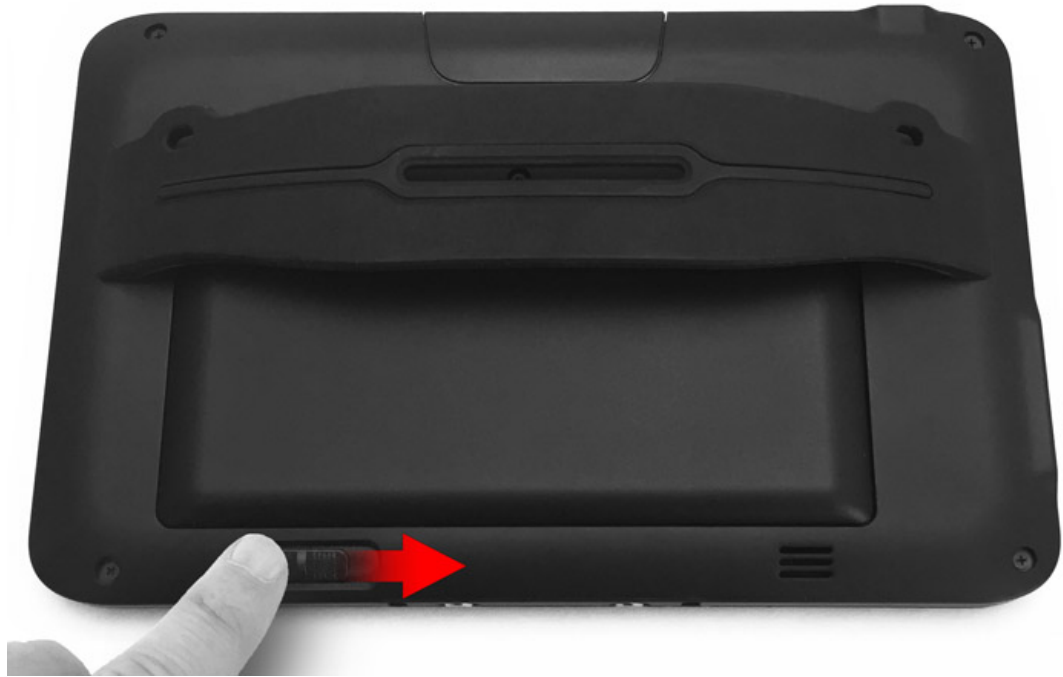
Figure 7-5 Removing the MICROS Tablet 720 Main Battery
