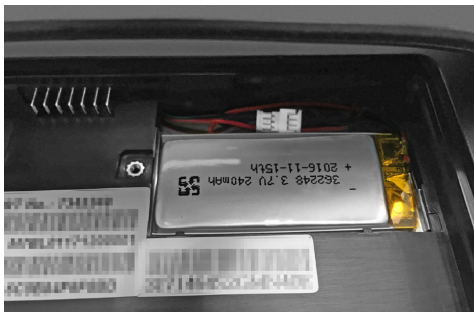
Figure 7-8 The Bridge Battery in the Battery Compartment
