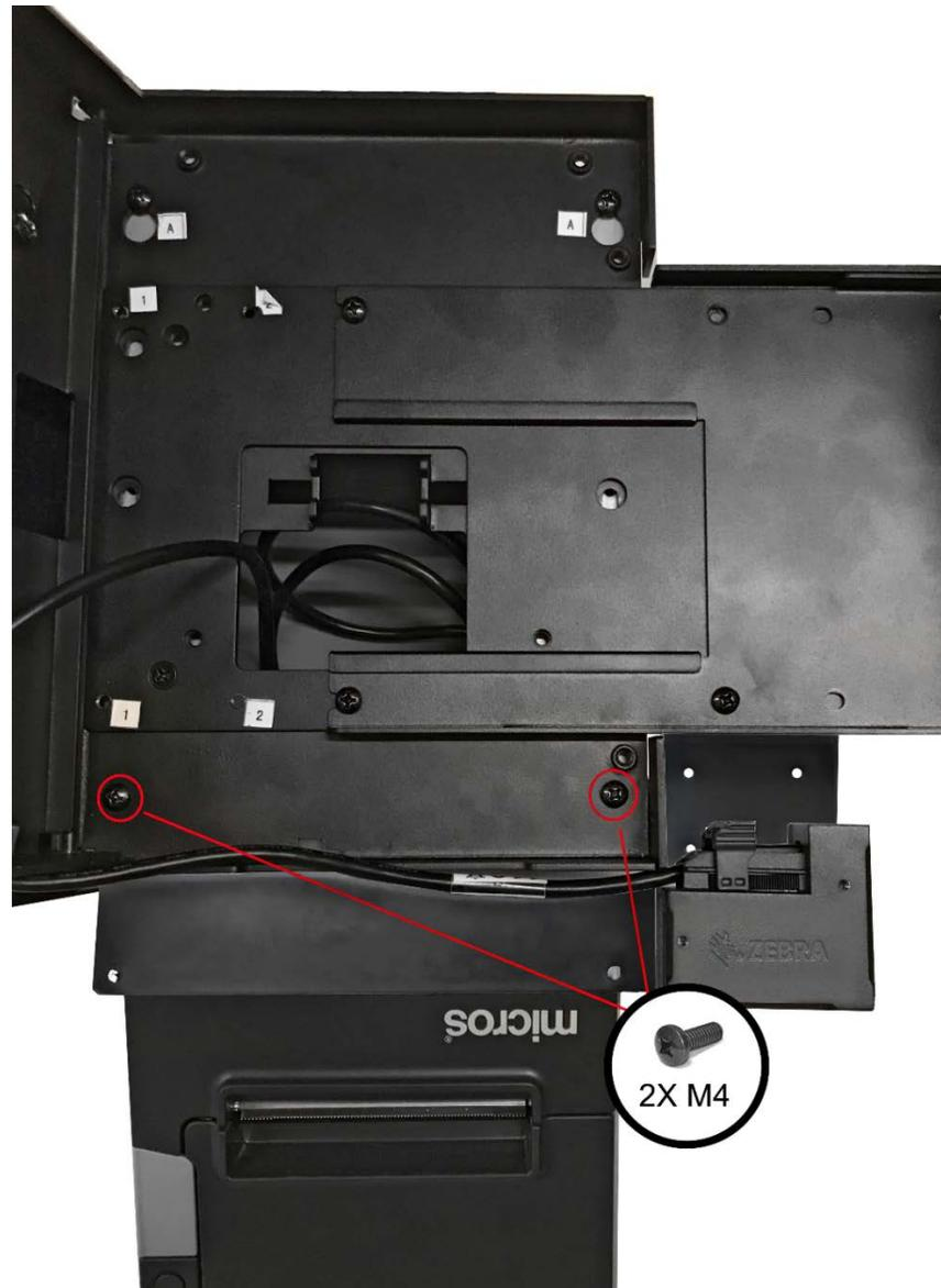
Attaching the scanner/L-bracket assembly to the floor head assembly. Image shows optional EMV cradle.
