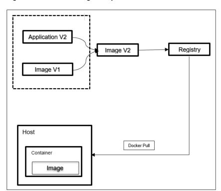
Figure 2-3 Modified Image Components
