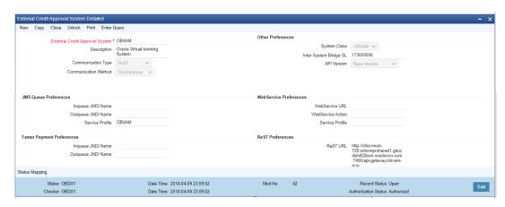
Communication Type should be 'ReST' and Communication Method should be 'Synchronous'
