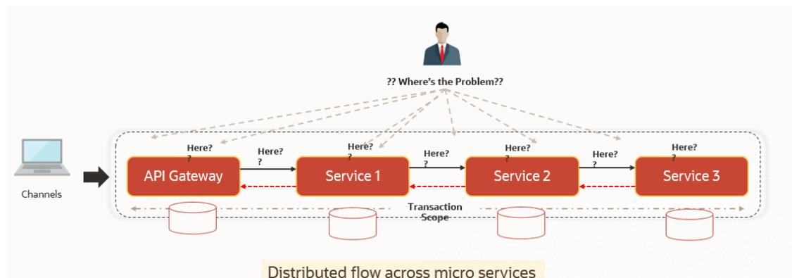
The [Figure 1-1](#) shows that it is important to establish the area of the problem on the service side. This can be achieved by a complete understanding of UI, Service side flows along with the data architecture of the application.
