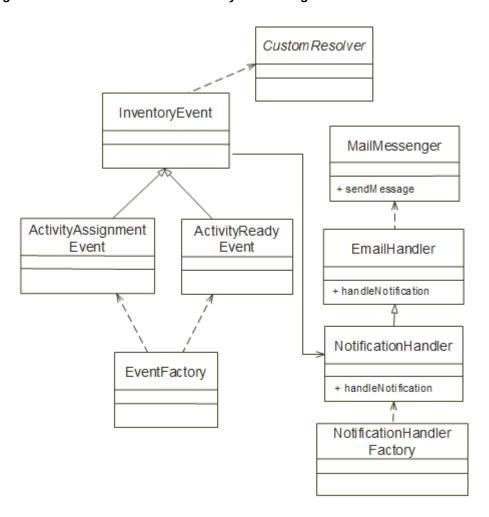
Figure 10-2 Notification Functionality Class Diagram
