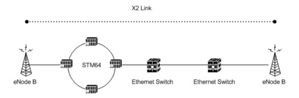
Figure 16-3 illustrates the **Connectivity Design** tab of this service connectivity. The service connectivity is enabled by five Ethernet connectivities, one of which is enabled by the STM64 ring.
