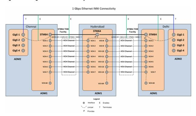
Figure 15-6 Gigabit Ethernet Enabled by VC4 Channels
