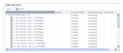
"Figure 17-16" shows how the Pipe Provides page lists all the child pipes that have been created based on the signal structure.
