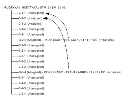
With these changes, a large contiguous block of channels becomes available, making it possible to assign them to the Ethernet pipe. Figure 14-25 illustrates these assignments.
