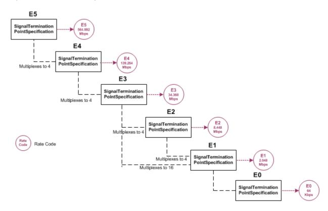
Figure 14-10 E-Carrier Signal Architecture
