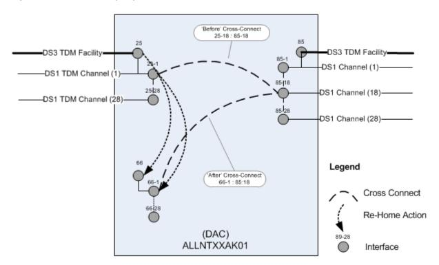
Figure 14-30 Rehoming Impact on Cross-Connects
