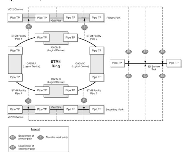
Figure 17-5 Multiple Enablement of an E1 Service Trail
