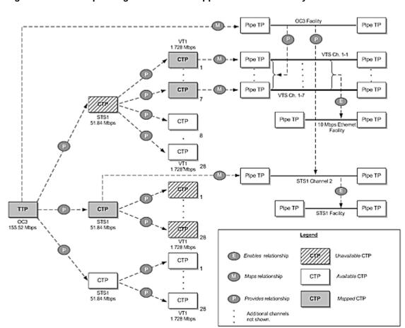
Figure 17-11 Complex Signal Structure Mapped to an OC3 Facility
