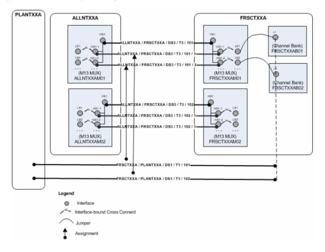
Figure 14-22 illustrates the results of the grooming activity. The channel reassignments have occurred. The new channels are terminated on a different MUX, so UIM has added cross-connects to join the interfaces on the MUX to the channel banks on which the T1s are terminated.
