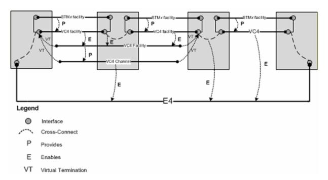
Figure 14-19 Virtual Termination on a VC4 Channel
