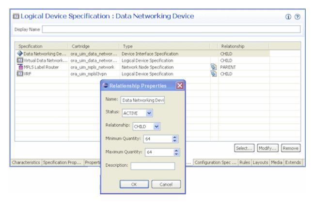
In UIM, when an entity is created based on the Data Networking Device specification, 64 device interfaces will be created based on the associated Device Interface specification. Because the maximum is set to 64, no additional device interfaces can be added to the logical device.
