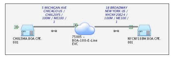
The service connectivity is enabled by UNI connectivities on the service location ends and network transport inside the service provider networks. Figure 16-8 illustrates the design of the service connectivity shown in the previous figures.
