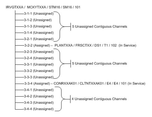
To free the required number of contiguous channels, the STM16 facility must be groomed. The channel assignments of the two E4 connectivities must be moved to make 7 contiguous channels available. The required changes are illustrated in Figure 14-24.
