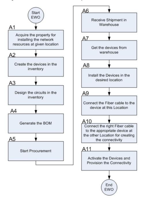
Figure 7-15 Access Site Workflow Template
