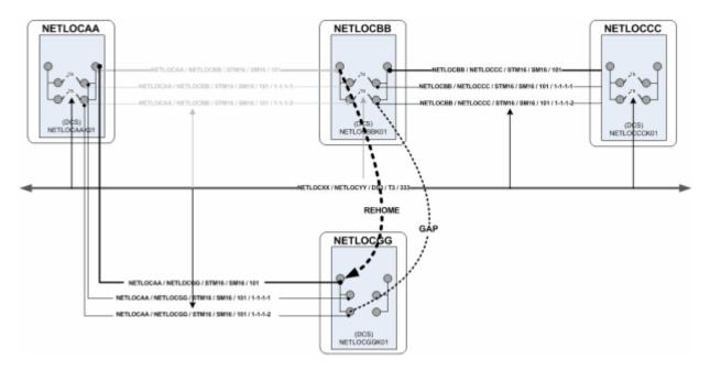
Figure 14-31 Rehoming with Resulting Gap
