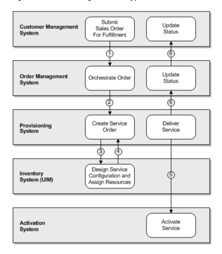
Figure 1-1 Provisioning Flow for a Typical Service Order
