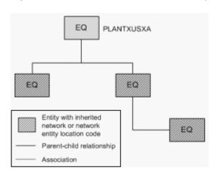
Figure 11-9 Network Location Code for Equipment Hierarchy
