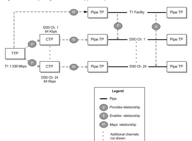
Figure 17-9 Simple Signal Structure Mapped to Pipes
