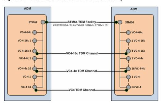
Figure 14-9 STM64 Channel and Device Interface Hierarchy
