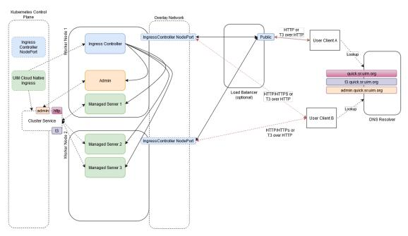
Invoking the UIM cloud native Helm chart creates a new UIM instance. In the above illustration, the name of the instance is "quick" and the name of the project is "sr". The instance consists of the WebLogic cluster that has one Admin Server and three Managed Servers and a Kubernetes Cluster Service.
