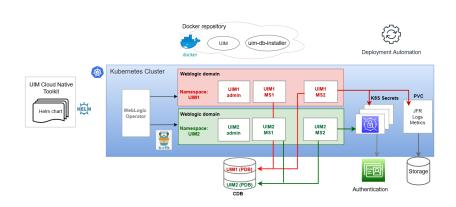
The UIM cloud native architecture requires components such as the Kubernetes cluster and WebLogic Kubernetes Operator, which are under your control to install and configure. A single WebLogic Operator can manage multiple UIM domains in multiple namespaces. Each domain is a dynamic cluster with multiple managed servers that is configured for integration with both optional and required components.
