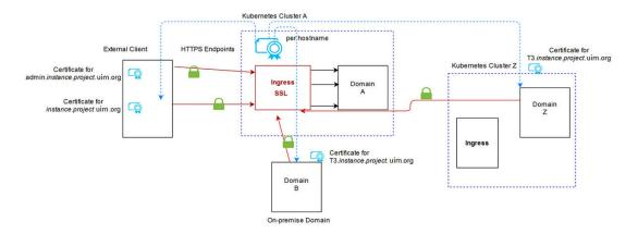
When UIM cloud native dictates secure communication, then it is responsible for generating the SSL certificates. These must be provided to the appropriate client. When a UIM cloud native instance in a different Kubernetes cluster acts as the external client (Domain Z in the illustration), it loads the T3 certificate from Domain A as described in "Configuring Access to External SSL-Enabled Systems".
