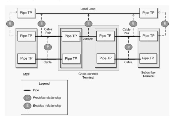
Figure 17-3 Pipe Relationships in a Local Loop Enablement
