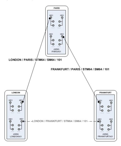
Figure 14-33 Simple Node Insertion Scenario
