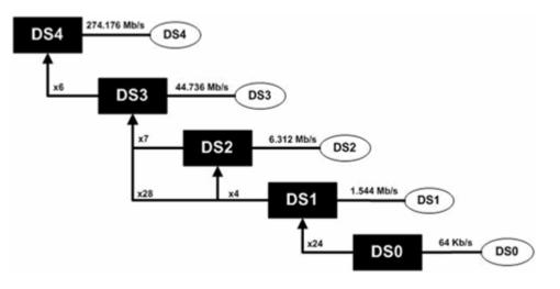
Figure 14-4 illustrates the hierarchy of channels that a connectivity requires to represent a T1 facility. The DS1 device interfaces on which the facility is terminated must include 24 DS0 sub-interfaces on which to terminate the channels.
