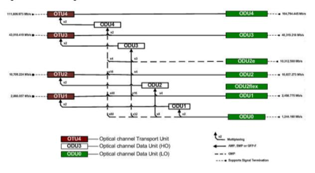
Figure 14-13 OTN Signal Architecture
