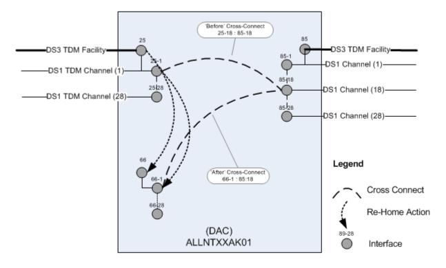
Figure 14-30 Rehoming Impact on Cross-Connects
