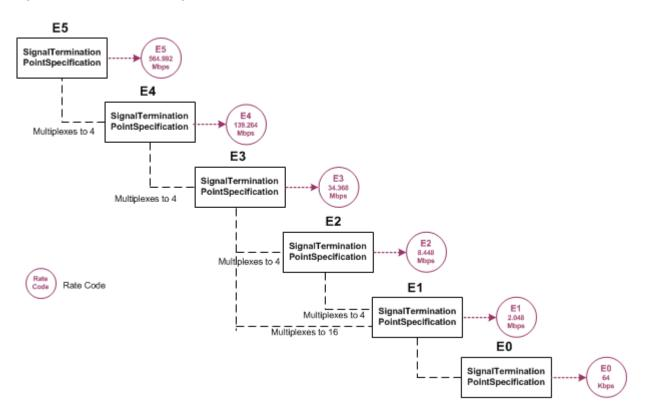
Figure 14-10 E-Carrier Signal Architecture
