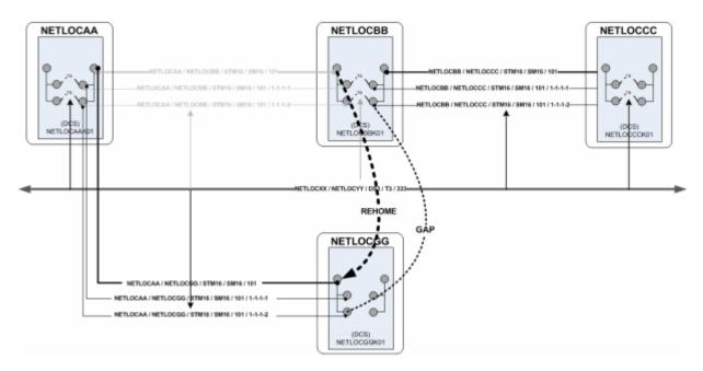
Figure 14-31 Rehoming with Resulting Gap
