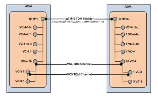
Figure 14-8 STM16 Channel and Device Interface Hierarchy
