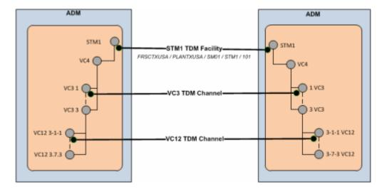
Figure 14-7 STM1 Channel and Device Interface Hierarchy
