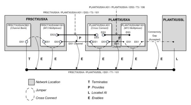
In this example, the FRSCTXUSXA / PLANTXUSSL / DS1 / T1 / 101 facility is terminated on a device interface in a channel bank located at the network location FRSCTXUSXA. Seven segments are required to complete the end-to-end connectivity path:
