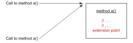
Figure 8-5, Figure 8-6, and Figure 8-7 show an extension point type of call, which dictates the extension point is weaved at the call to the method defined by the extension point. For this
