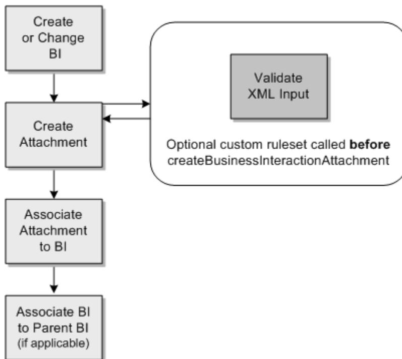
In Figure 2-2, the **Validate XML Input** box represents the custom ruleset that you can configure to run before the creation of the attachment. See "Validating Input Data" for more information.
