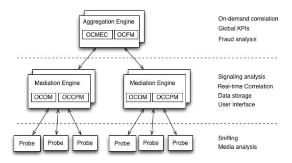
Each of the three layers supports high-availability by deploying two identical servers in active-passive or active-active modes of operation. For small setups, it is possible to run the probe layer and the ME layer on the same physical hardware. The AE layer always requires its own hardware.
