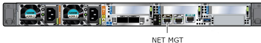
Figure 3-4 Connecting to ILOM over the Network
