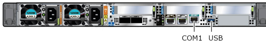
Figure 3-3 Connecting to USB and SER MGT (COM1) Ports
