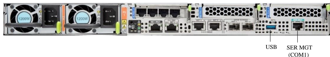
Figure 2-14 Connecting to USB and SER MGT (COM1) Ports
