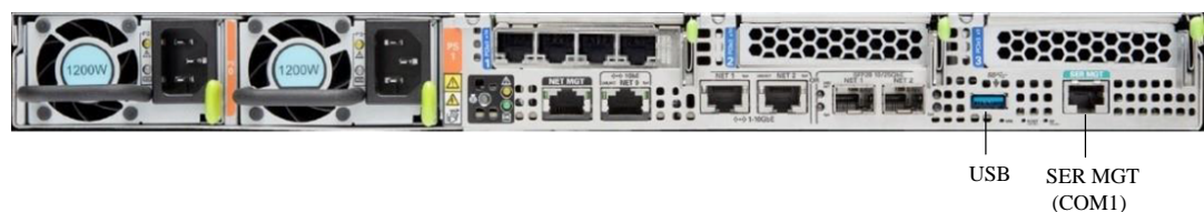
Figure 4-14 Connecting to USB and SER MGT (COM1) Ports
