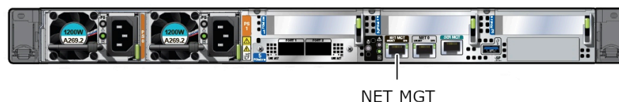
Figure 5-14 Connecting to ILOM over the Network
