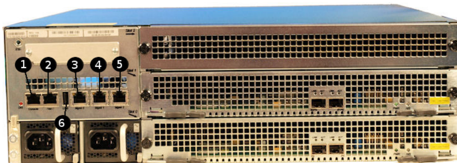
Figure A-6 Acme Packet 6300/6350 Management Interfaces
