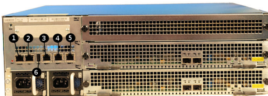
Figure A-5 Acme Packet 6300/6350 Management Interfaces
