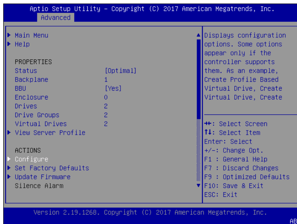
Figure 3-2 Begin RAID Configuration
