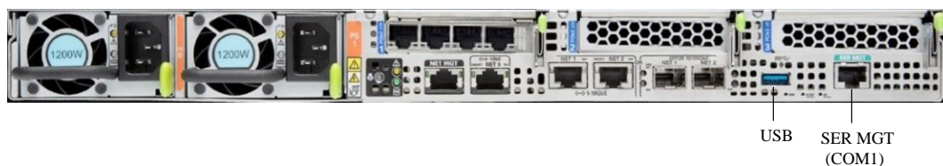
Figure 3-14 Connecting to USB and SER MGT (COM1) Ports
